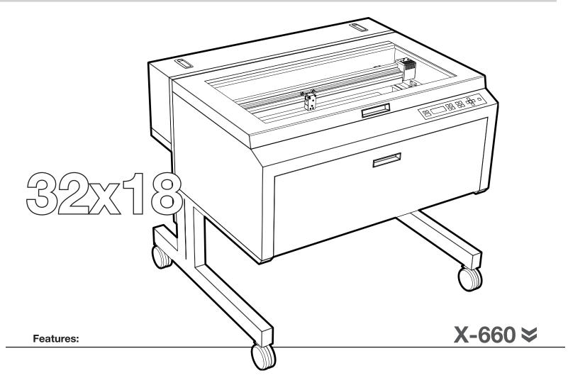
Free-standing unit with integrated cart,motorized Z-axis, auto focus, X-Y beam positioning system with RACER™ motion technology, self adjusting spring loaded sealed bearings, stationary processing table, Quick Change Laser Cartridge™ shielded optics, interchangeable focusing optics, flash upgradeable electronics, job complete indicator, system status indicator, relocatable origin, enhanced vector cutting, 3D engraving and rubber stamp mode.
